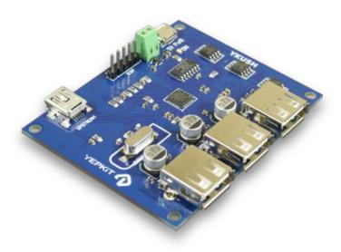
To address this issue, YKUSH provides to the user the capability, through software, to selectively turn ON and OFF each of the USB devices connected to the hub.
