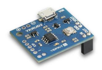
It's a compact board designed to be easily integrated together with the Raspi board.
